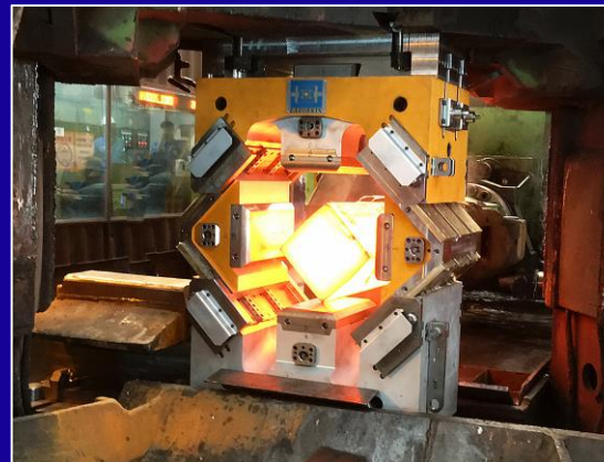
With system to quickly fix FDFD to the top die
