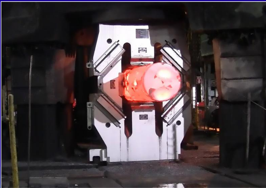
FDFD with dies to produce the forgings with round cross-section
