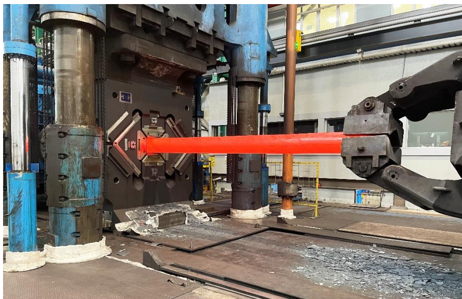
Fig.12 – Calibration forging using FDFD
