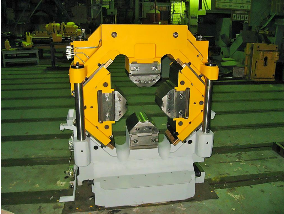
Fig.6 – Design of FDFD with guide posts and metallic springs
